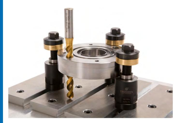
Quick setting with the clamping bolts: move each single bolt without clamping screw into the slide block of the machine table and position the bolt by hand as a stopper at the workpiece. Tighten the clamping bolt and it automatically helps you to position the workpiece.
