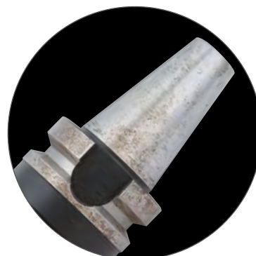
通常他社品サビ発生面 Rusted surface of standard product
