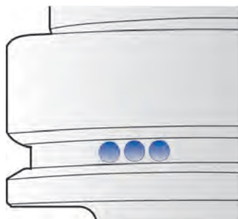
Fine-balanced with balancing bores in the flange
