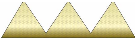
Figure 2: Grain structure of cut thread
