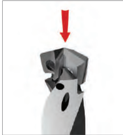
Step 2: Slide the insert into the precision ground locating pocket on the holder. The insert should not be turned, rotated, or twisted for locking purposes. The holder pocket and locating pads on the insert assure optimum fit and repeatability.
